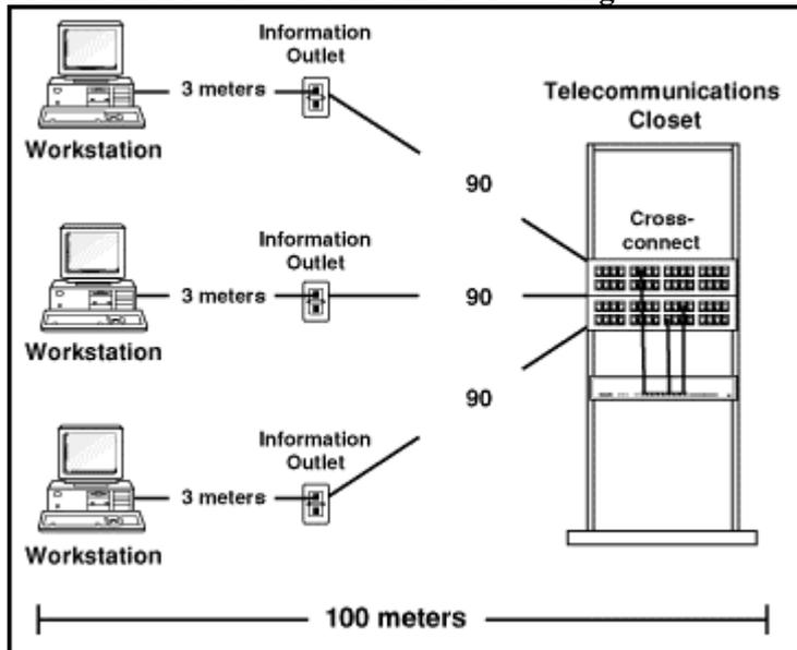
In addition to the 90 meters of horizontal cable, a total of 10 meters is allowed for work area and telecommunications closet patch and jumper cables.
